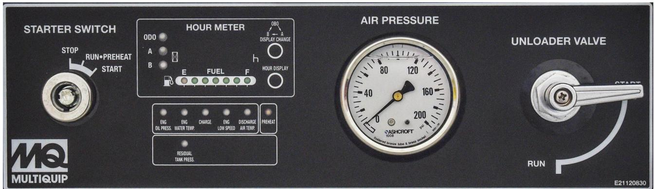
**Control Panel** monitors compressor and engine statistics:
